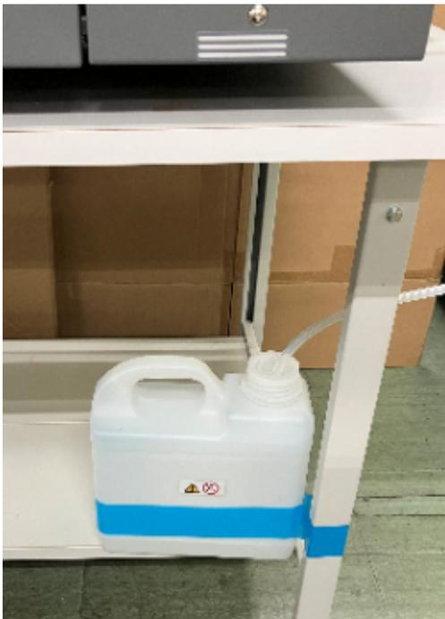
**IMPORTANT!** Install the waste ink bottle vertically. If installed horizontally, the waste ink inside could leak out.
