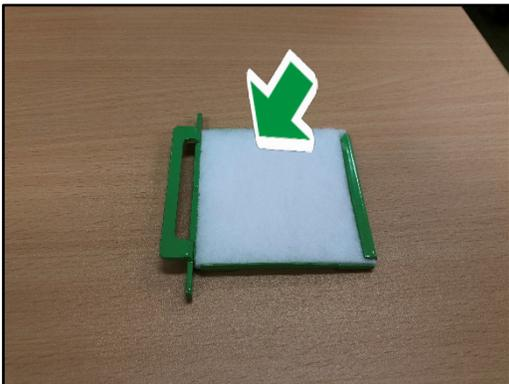
7. Insert the mist fan filter fixing frame into its original position until it clicks.
