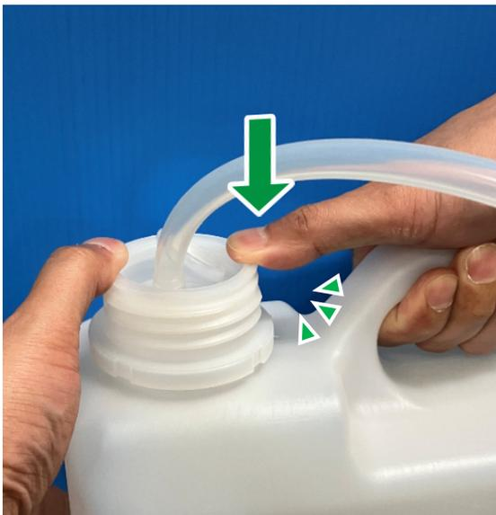
Close the waste ink bottle cap tightly and make sure that there is no gap between the waste ink bottle cap and the waste ink bottle.
