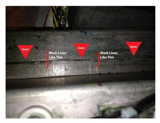
After marking this edge, remove the 4 screws holding the maintenance station assembly to the base. Once the 4 screws are removed, you will be able to lift the maintenance station off the base. See picture below.
