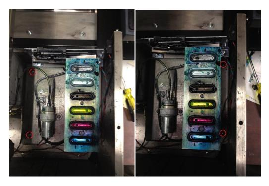
Once you take the maintenance station off its base, you must remove the 5 wires plugged into the board located underneath the maintenance station. You also want to disconnect the drain tube from the waste ink tank. See images below.
