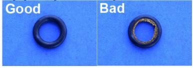
If you are not able to draw ink with the damper on but were successful with the damper off, the damper is damaged or clogged and will need to be replaced.
