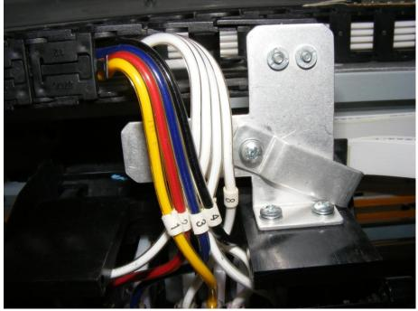
Unclip 3 to 4 links from the tube carrier and take the print carriage lid off.
