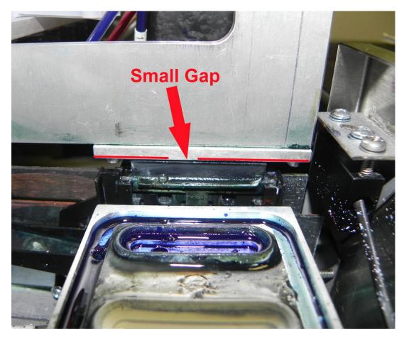
• Look at the print head carriage from the front; you will notice that the bottom plate has a small ramp to it before it turns flat on the left hand side. The wiper blade should start to touch the bottom of the plate around the middle to upper middle of the ramp area.
