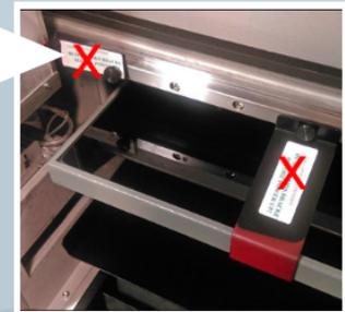
**IMPORTANT:** The 2 retainer brackets and 3 thumb screws must be removed before use. Keep them for later use
