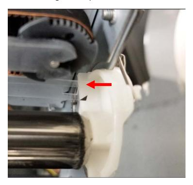
12. Secure the encoder strip from the hook on the right-hand side of the printer
