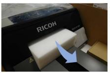
Table in printer is secured by Foam block. Please remove before startup
