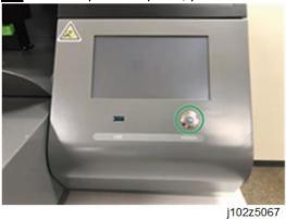
**13.** After the printer turns on, the printer will go into a initialization and boot up routine the it will begin charging with ink.
