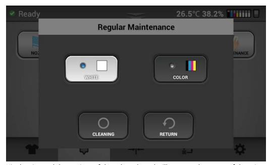
Hit cleaning and the carriage of the color selected will move to the center of the printer.
