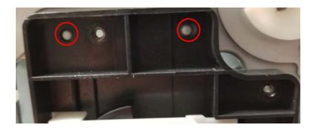
Now you can install the two screws to secure the maintenance station.
