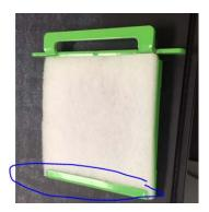
Make Sure when putting the filter and holder back in the printer the square opening is pointing up towards the top of the printer (nod the round opening in the holder). This will make the orientati on of the green handle towards the top of the printer. If it is installed in the reverse (round opening pointing up) then the handle will be too low and the carriage will hit in causing and er ror and possible damage to the printer.
