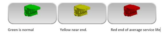
Note: The printer will still function even after parts have exceeded their service life although it is highly suggested that the part be replaced as the part may fail soon which may lead to other part failures – This is true EXCEPT for the INK sumps - the ink Sumps must be drained when they have reached 100% as the machine will not be able to print or conduct auto maintenance.
