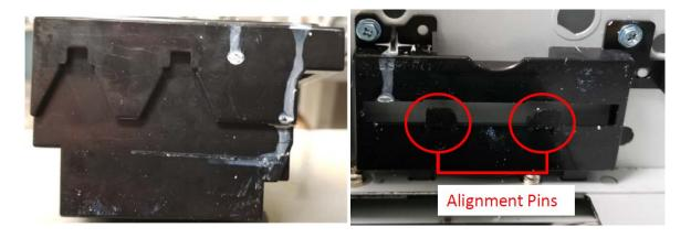
Make sure the sump is installed correctly and is not crooked as this can cause nozzle problems. Now install the maintenance unit.
