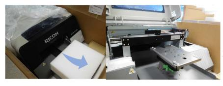
Hold foam block on the side and gently pull forward. With block removed, continue with set up steps as described in the **user manual**.
