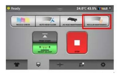
Select which maintenance unit you will be cleaning based on the frequency
