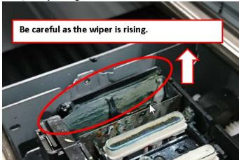
Step 9 Wipe away grease that protrudes far beyond the coverage of Fig. 1, 2 and 3. Also, confirm that grease is not attached to the Filler Sensor.
